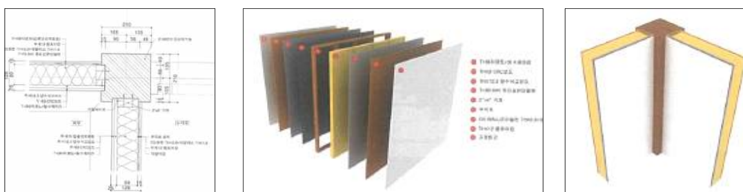
New Hanok Construction Technology – Wall Connections
